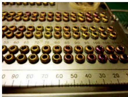
Fig. 3: Discolorations caused by oxidation
